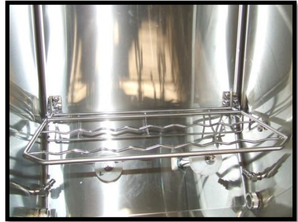
BOWL RACK MUST BE IN DOWN POSITION
