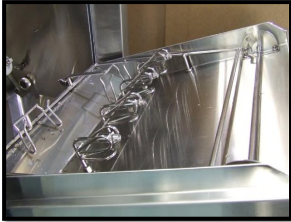
BEDPAN RACK MUST BE IN THE DOWN POSITION
