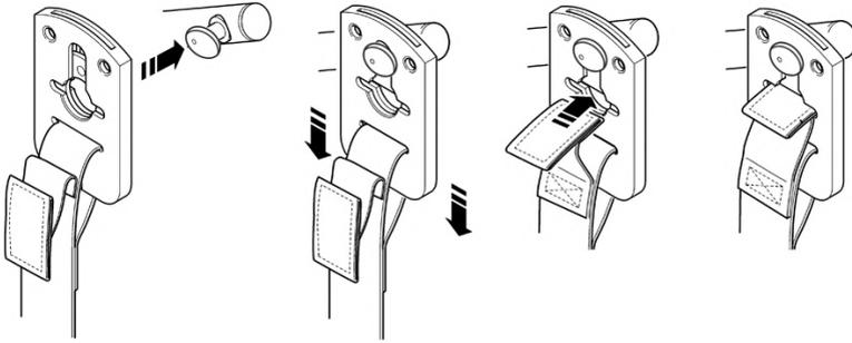
**Securi3 sling attachment system.** Example of installation.
