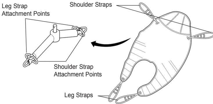
**6-point spreader bar.** Example of 6-point spreader bar sling with loop attachments.
