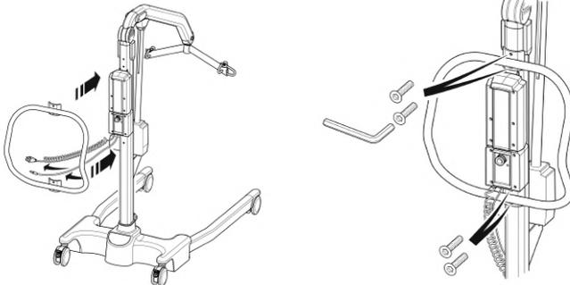
6. Fit power pack to the lift and make sure the latch holding the pack in place is fully engaged. "Click" in place.
