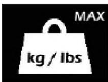
If the lift stops because of an overload (an attempt to lift more than the safe working load) the overload symbol will appear on the LCD display and the lift will cease to operate until the additional load (above the SWL) has been removed.
