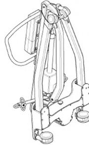
2. Release the leg and mast assembly by unfastening the restraining strap from the wheels. This strap will retract neatly into the top of the mast section.
