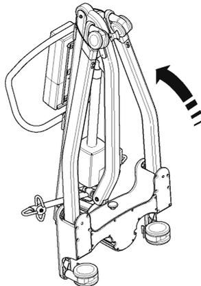
5. Pull the restraining strap sharply upwards and extend over the wheels. (This will keep the legs, mast and boom neatly together during transit and storage).
