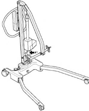
2. Release leg-locking device (pulling it away from the cast base), close legs tightly together.
